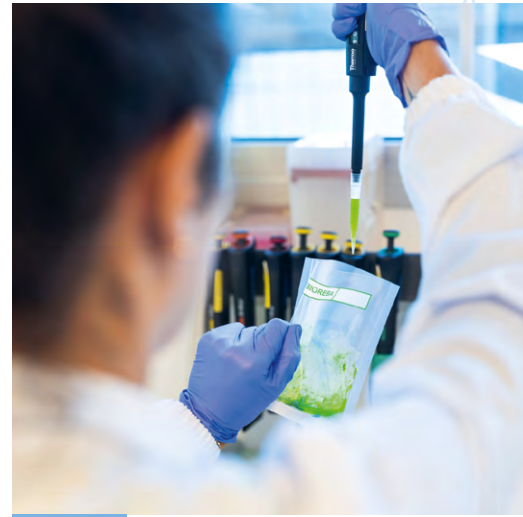
Test sample taken from banana leaf homogenate for the detection of plant pathogenic viruses using the ELISA serological technique.
